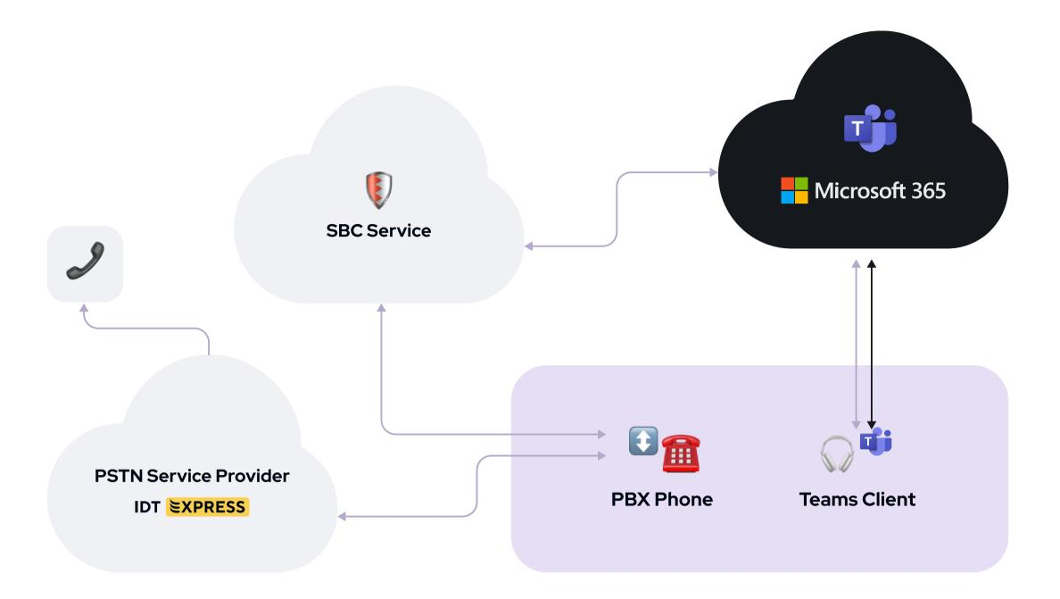
With station-side integration, all the calls go through the PBX, and users can call anyone internally simply by dialing an extension. The PBX can send calls directly to Teams users, making this configuration ideal for Teams Calling provision to a limited set of users.
