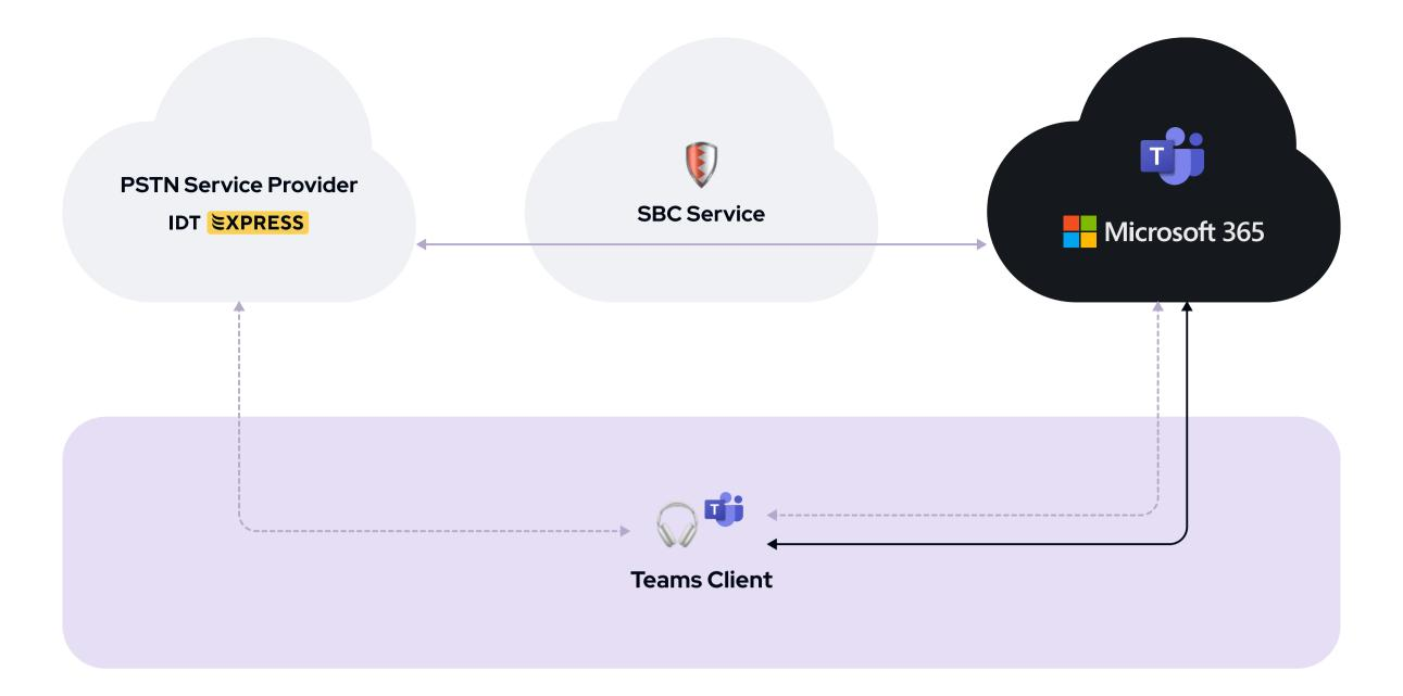
Here, your communication service provider (CSP) will connect directly to the Microsoft 365 cloud hrough a cloud-based SBC. This Session Border Controller may be one that your organization owns, and deploys in the cloud through a commercial platform such as Azure or AWS. Alternatively, the CSP itself may own, host, and manage the Session Border Controller.
