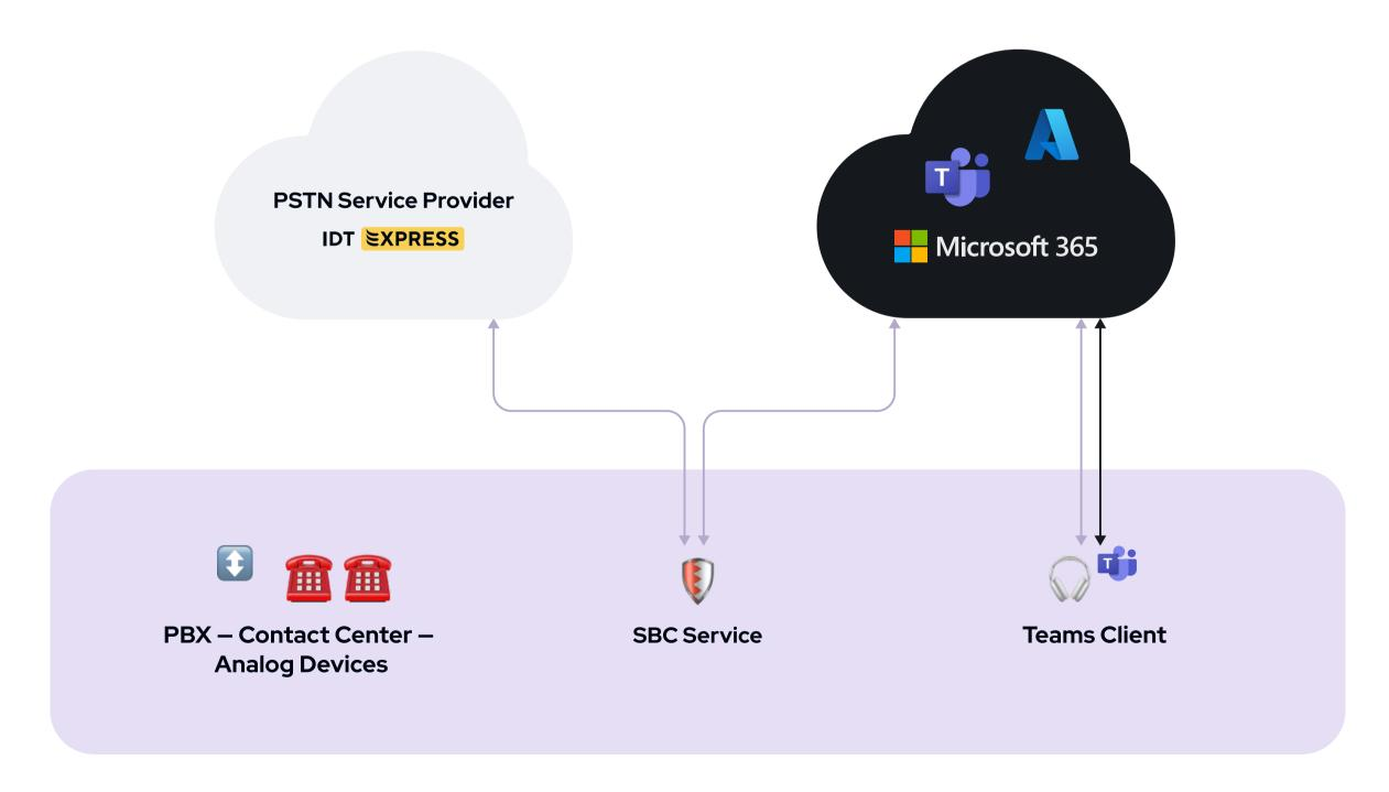
Here, calls move in and out of the system through an on-premises SBC which is connected to your organization's communication service provider, and to the Microsoft 365 (Azure) cloud. Note that there may be considerable costs involved in maintaining legacy communication devices and infrastructure. In the long term, it may be more cost-effective to consider upgrading to a fully digital infrastructure and cloud-based deployment model.
